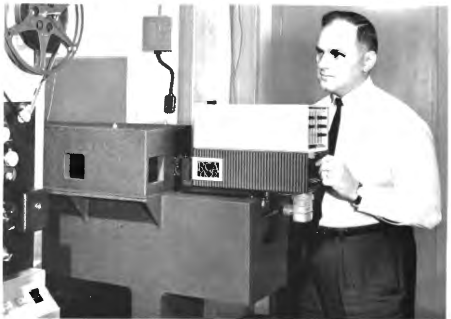
FIG. 2. TK-22 Camera installed on a TP-11 Multiplexer. Complete set-up adjustments can be made from this location.
