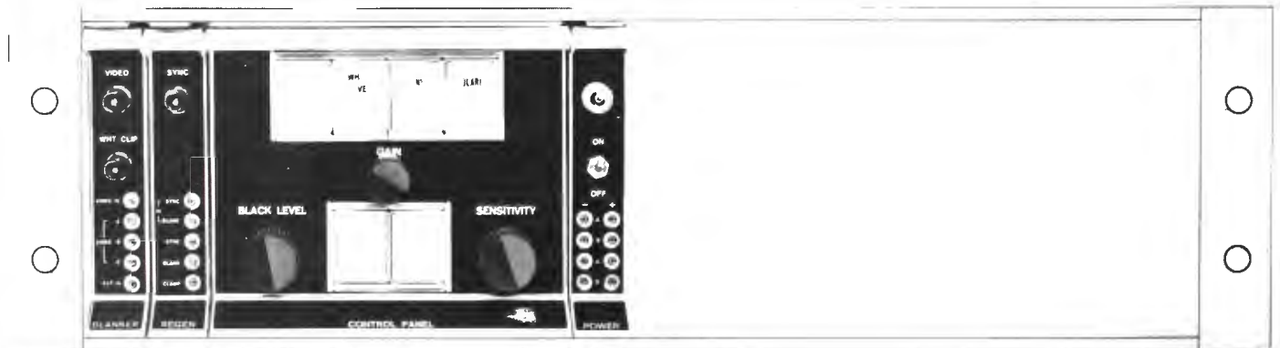
FIG. 7. Closeup of the auxiliary equipment used with the TK-22 Camera. A remote control panel is located at this position.
