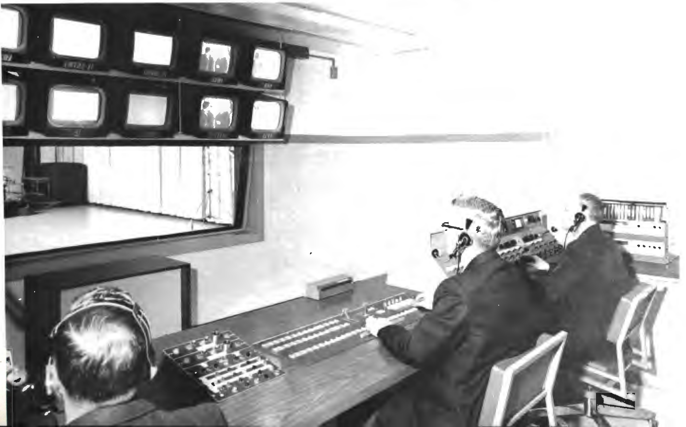
FIG. 17. Control for Studio "A" (shown) is identical with Studio "B". Both feature TS-40 custom-built switchers with special effects. Note transistorized audio control at right.
