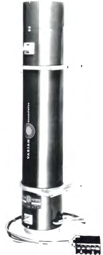
FIG. 16. High gain TWT (traveling wave tube) used in driver stages of new RCA 10- and 2-kilo-watt UHF transmitters.
