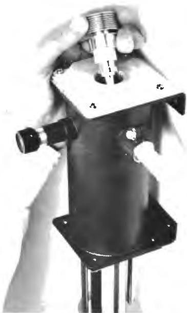
FIG. 5. Identical ceramic 7289 tetrodes and tuned cavities serve as IPA's for aural and visual channels of 30-kw and 50-kw transmitters. Stages occupy upper half of left-hand cabinet.
