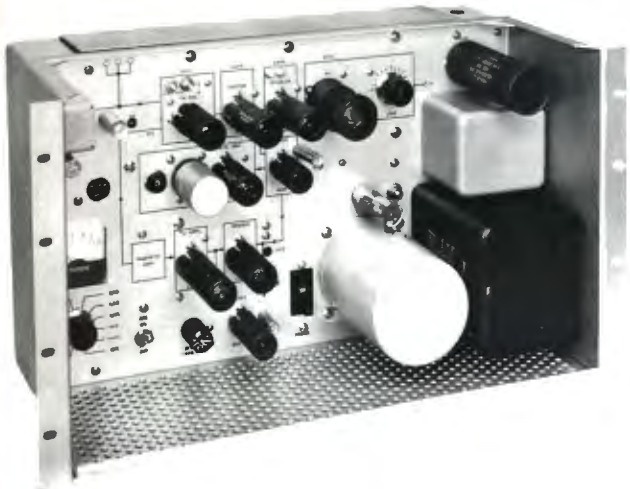
FIG. 24. BTE-10C Direct FM exciter used in all RCA UHF-TV and RCA high fidelity FM transmitters.
