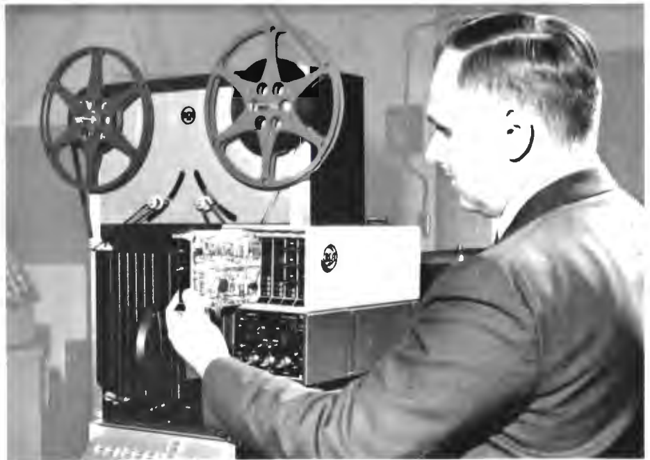
FIG. 3. Camera modules are of the standard plug-in type and interchangeable with many of those used in new live and film color cameras.
