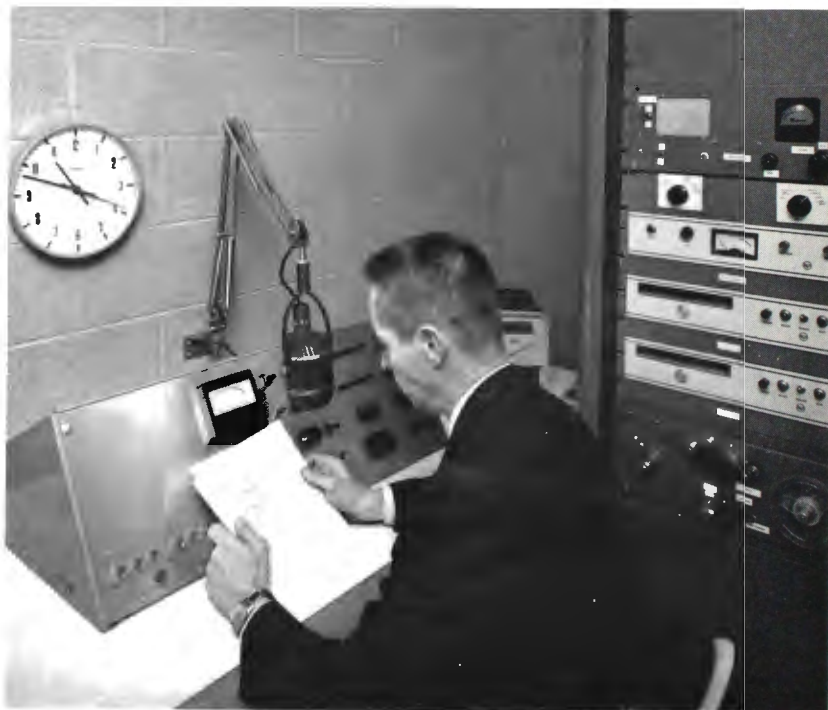
FIG. 20. News Broadcast Booth. Here the seven mobile units can be contacted and reports may either be put on-air "live" or recorded. (Newsmen use hand-carried 2-way radio units for places not accessible to regular mobile units.)
