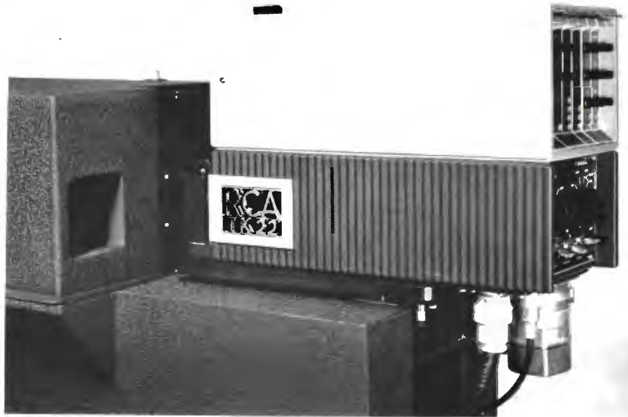
FIG. 1. Small size and low power consumption allows concentration of circuits at the camera head position.
