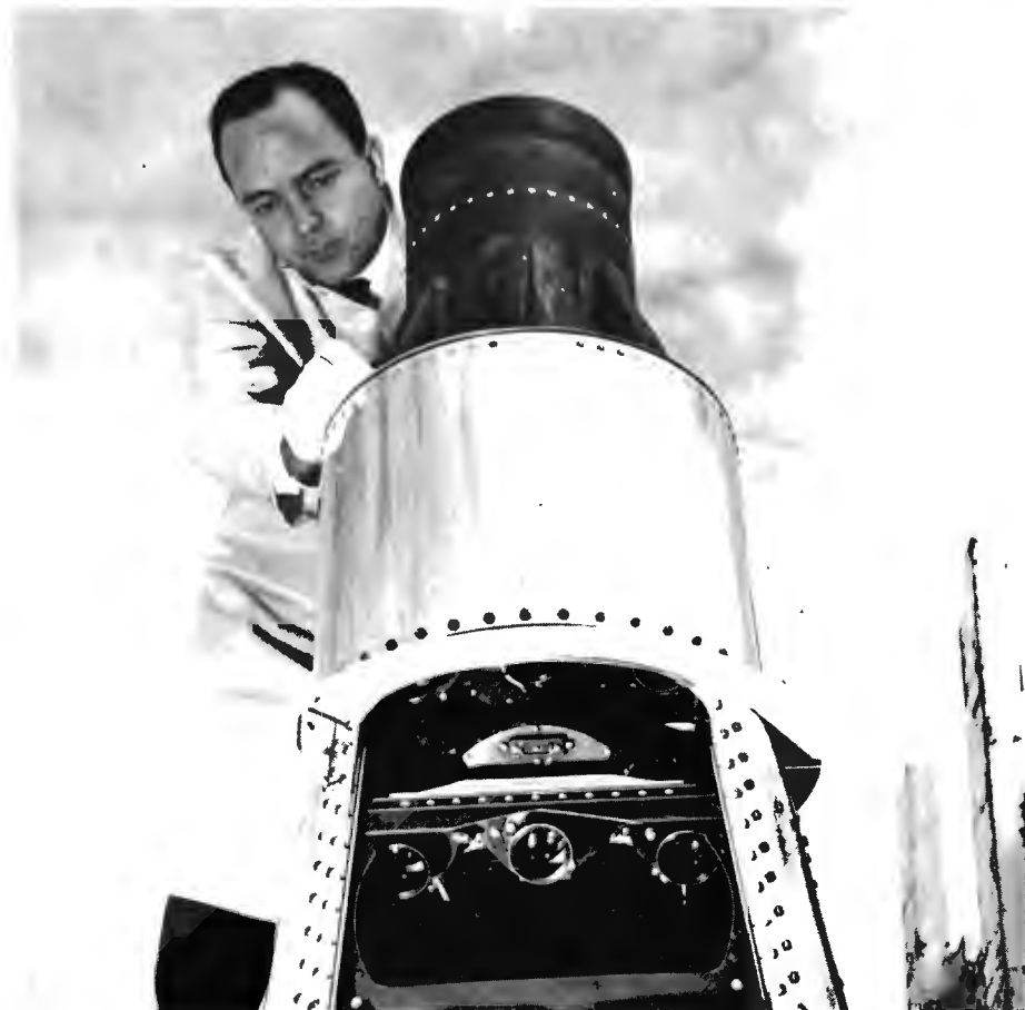
TV cameras peered at moon from this aluminum shroud, shown by Ernest Toth, RCA technician.
