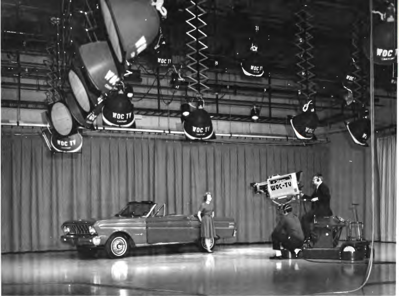
FIG. 29. Studio "A" includes 18-foot turntable with two mikes and a-c outlets. It will run up to 2½ rpm in either direction.
