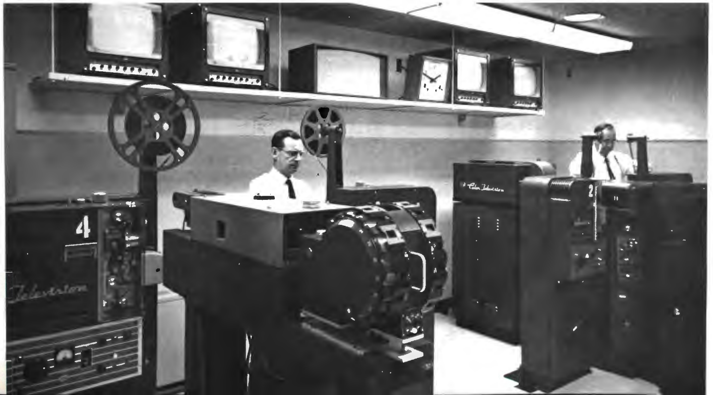
FIG. 33. Two islands of film equipment at WOC. Each is equipped with two film projectors and a slide projector. Island at left handles black and white. Island at right handles color as well as black and white.
