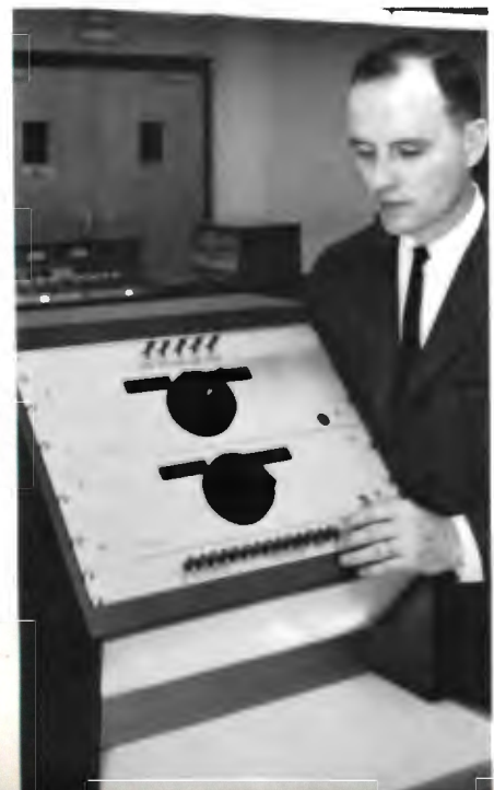
FIG. 25. Chief engineer David Hauser at custom-built delegate control in projection room. Top switches operate intercom. Upper large switch delegates film projectors and slide projector on TP-11 island to "A", "B", or Master Control. Lower large switch delegates projectors and slide projector on TP-15 (color) island to studio controls. Bottom row of push buttons is WOC house monitoring system, to punch up any of 15 video sources with matching audio.
