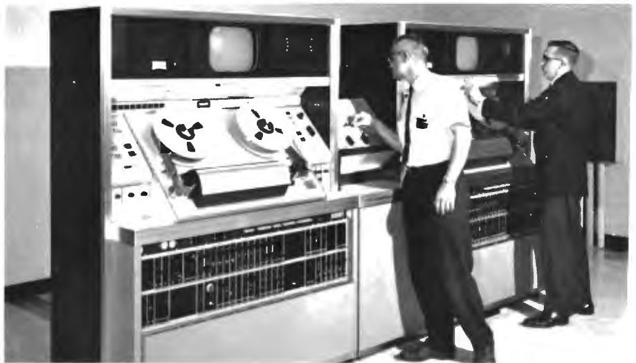
FIG. 28. Special TV tape delegate control was designed and built for WOC. Note that housing blends with RCA tape recorders.
