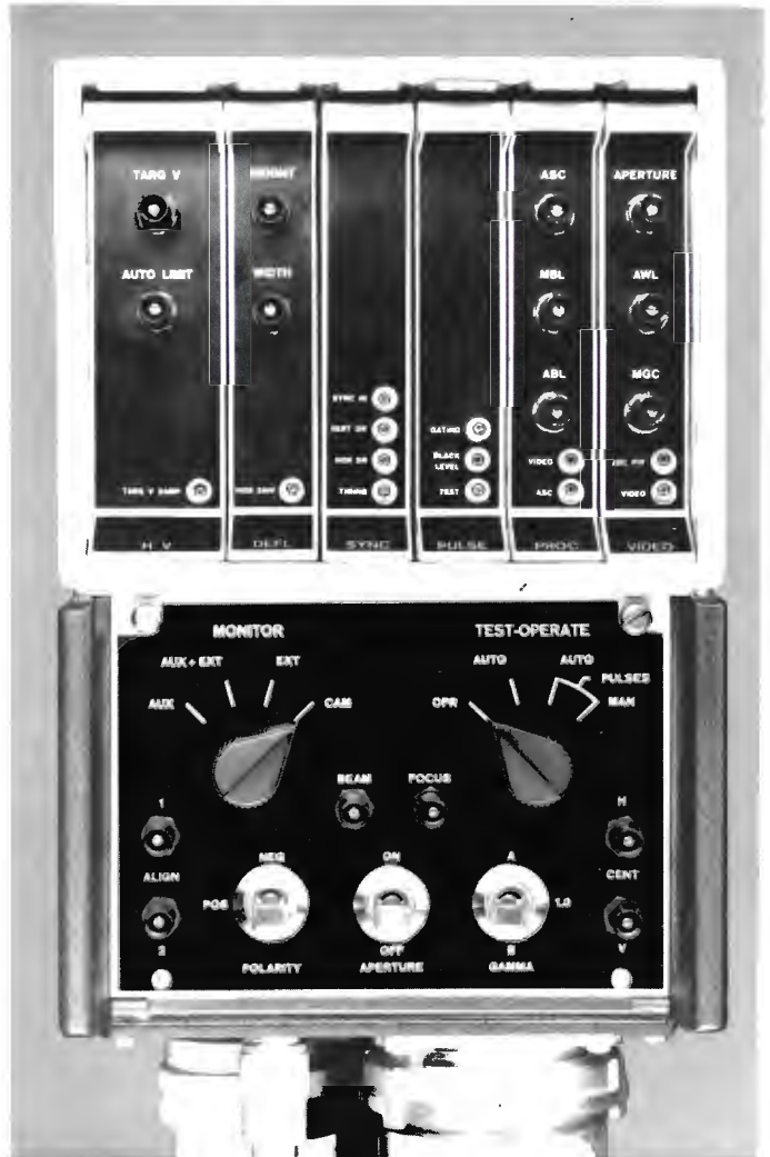
FIG. 3. Camera modules are of the standard plug-in type and interchangeable with many of those used in new live and film color cameras.
