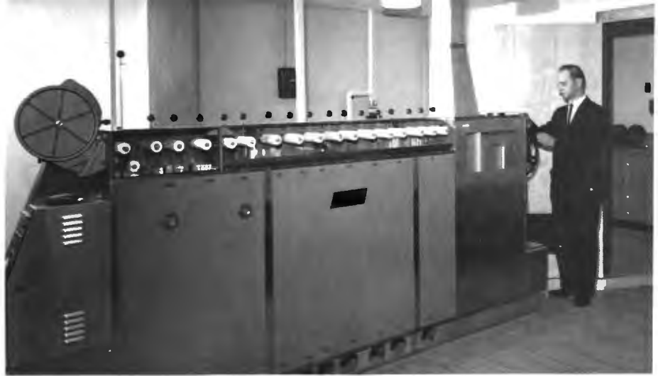
FIG. 21. Houston Fearless 16mm reversal film processor is part of News Dept. facilities. Dark room adjoins the processing room.
