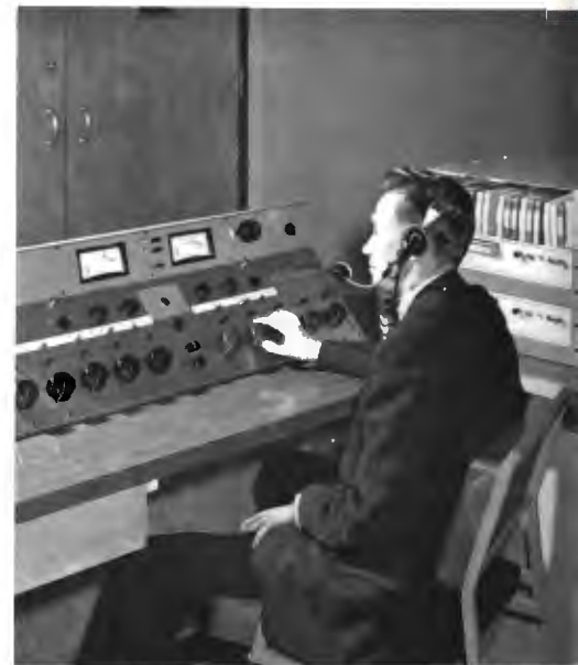
FIG. 30. One of three BC-7 transistorized audio consoles in new WOC. This is sub-control B. Included are two cartridge tape units and turntable.
